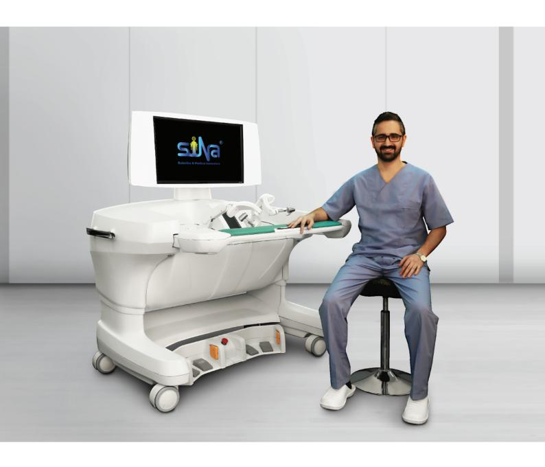
Sina<sub>flex</sub> is a robotic surgery system which can be used for performing abdominal surgery operations in an ergonomic posture for surgeon and also remotely through internet or other communication channels. This system has two main subsystems including a master robotic console at the surgeon's side and a slave robotic system at patient's side.
